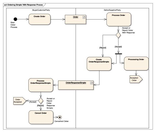
Figure 2, The OrderingSimpleR process.
